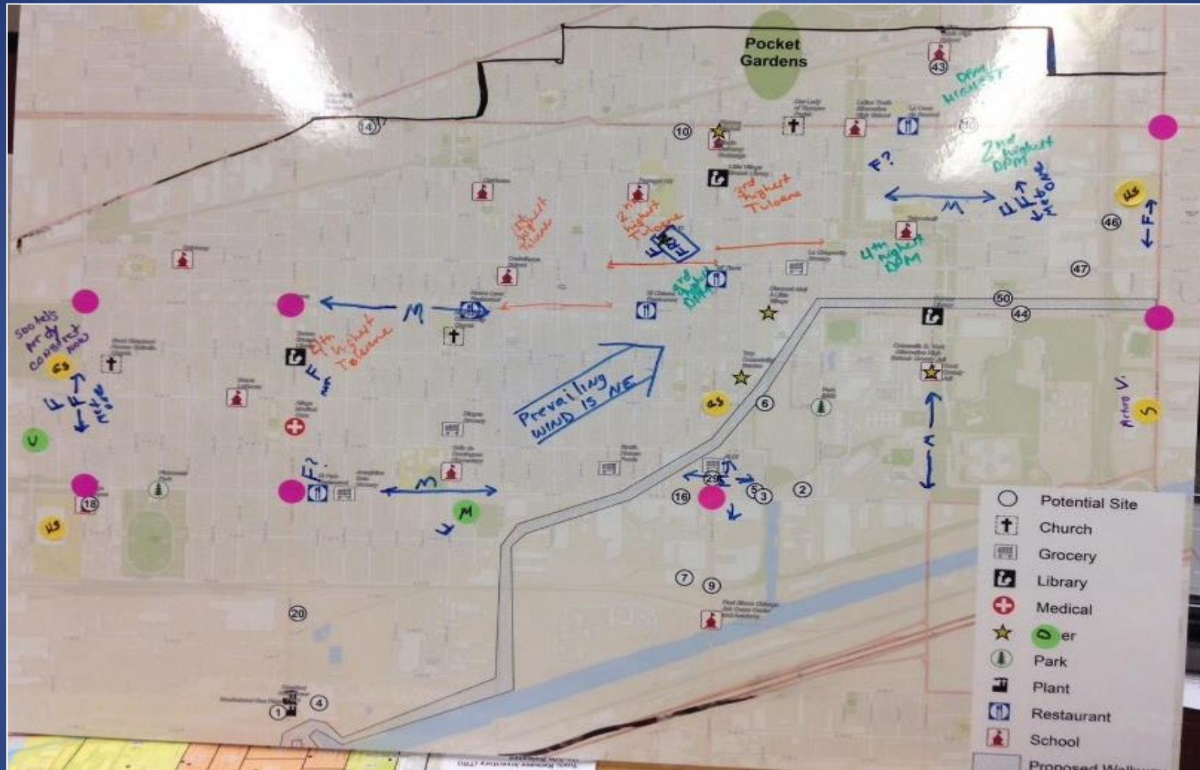
F: Fixed air monitoring sites; M: Mobile routes; Pink Dots: Intersections/Roadways of concern to community; Green Text: Tiers of DPM concentrations (high to low); Orange Text: Tiers of toluene concentrations (high to low)
