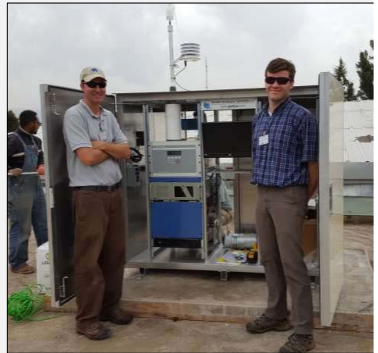
An U.S. embassy air quality monitor system with a BAM inside a shelter.
