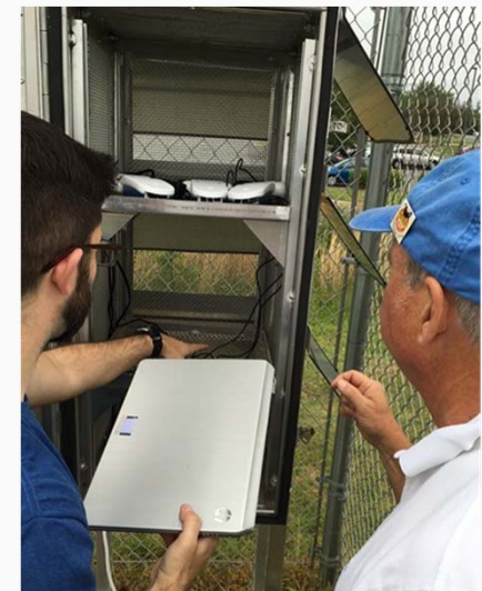
CAC staff and citizen volunteer checking on ozone sensors at deployment site
